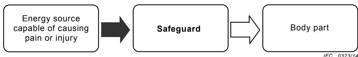
Figure 2 – Three block model for safety
