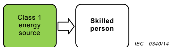
Figure 16 – Model for protection of a skilled person against a class 1 energy source
